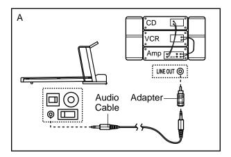
B. Plug one end of the audio cable into the jack on the front of the treadmill near the power cord. Plug the other end of the cable into the included adapter. Plug the adapter into an RCA Y-adapter (available at electronics stores). Next, remove the wire that is currently plugged into the LINE OUT jack on your stereo and plug the wire into the unused side of the Y-adapter. Plug the Y-adapter into the LINE OUT jack on your stereo.
